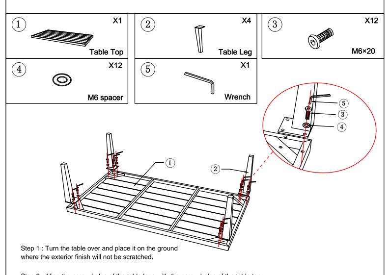
Step 2 : Align the screw holes of the table legs with the screw holes of the table top, insert flat washers(4) and screws(3) into each hole, once the screws are in place, tighten the screw until firmly attached with the wrench provided.
