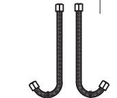
4. Screw spray hose to the copper pin (the longest pin). Make sure to have a tight seal using adjustable wrench. Attach supplied counterweight to the hose.
