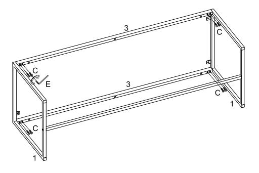
Secure part (3) to part (1) using bolt (C) with hex key (E).
