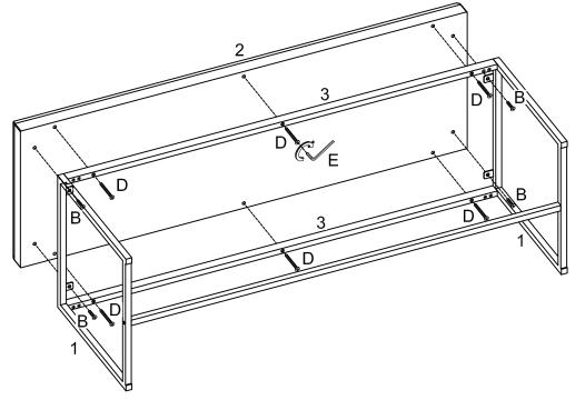
Attach part (2) to part (1,3) using bolt (B,D) with hex key (E).
