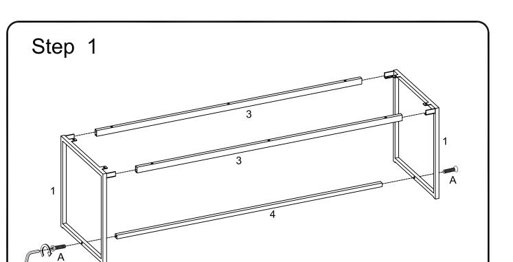
Attach part (3,4) to part (1), secure part (4) to part (1) using bolt (A) with hex key (E).
