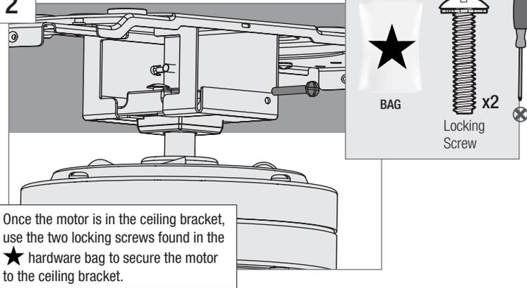
Once the motor is in the ceiling bracket, use the two locking screws found in the ★ hardware bag to secure the motor to the ceiling bracket.
