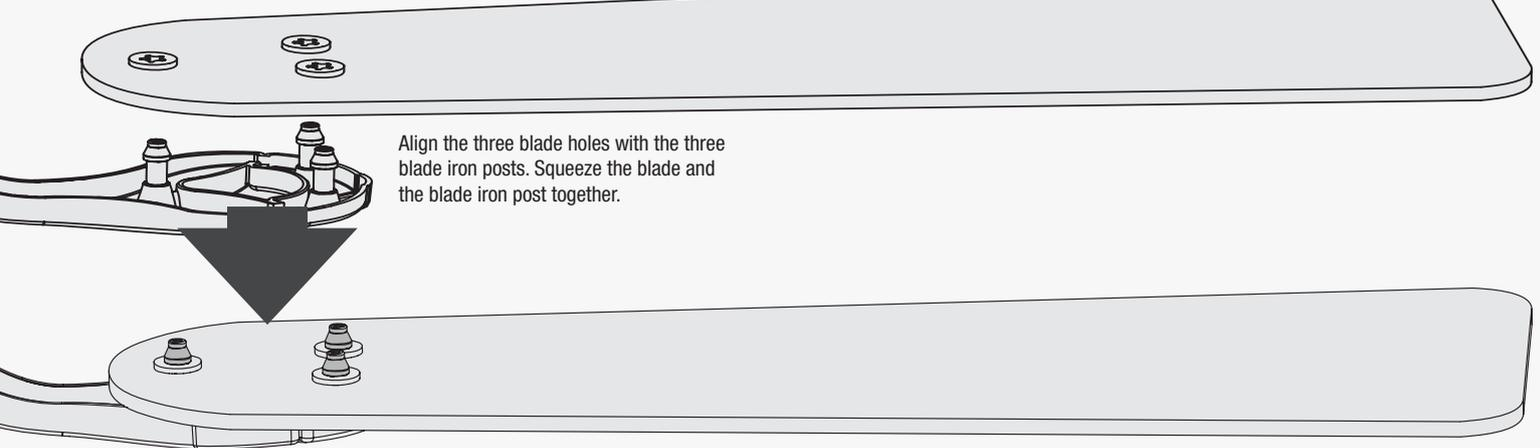
The flared tops of the blade iron posts will be fully visible above the blade when properly assembled.
