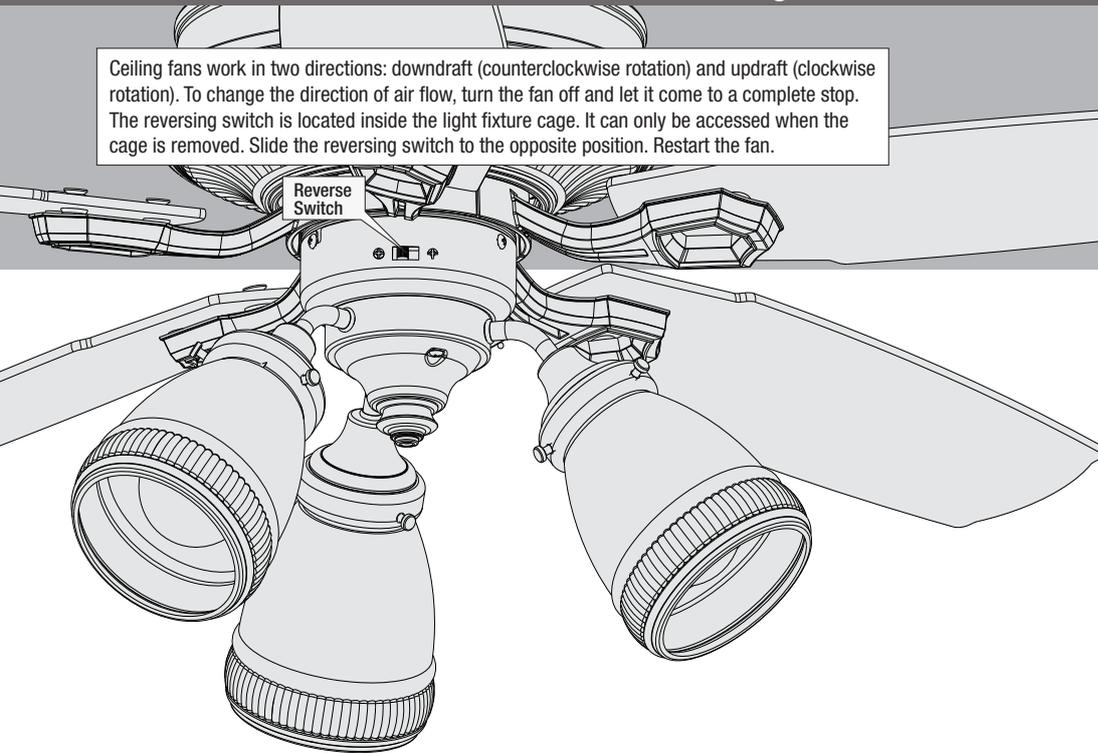
Updraft (clockwise rotation) creates a more indirect airflow. Updraft airflow is great for moving warm air downward.
