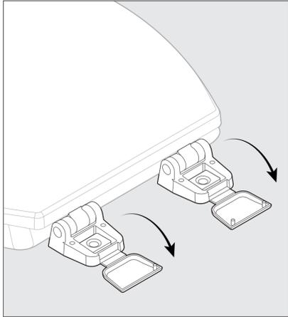
(2) Insert plastic screws into the holes of the hinges
