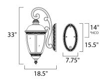
\*height from the top of the fixture to the center of the outlet
