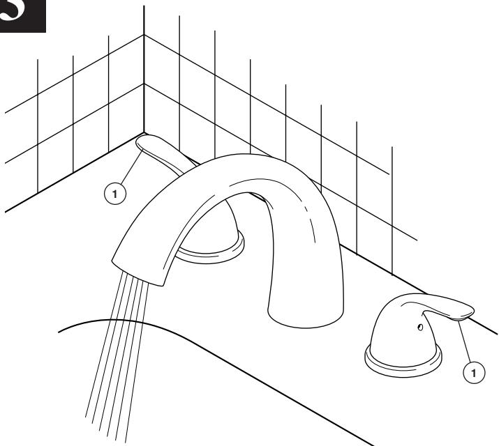
Turn faucet handles (1) all the way on. Turn on hot and cold water supplies and flush water lines for one minute.
