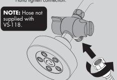
Thread other end of Hose onto base of Handheld Shower. Ensure sealing washer is inside Hose end to avoid leaks. Hand Tighten connection.
