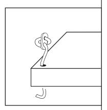
Installer Tip (1): It is recommended that two installers are required to adjust the height of the fixture. One installer to hold the fixture, and the second installer to adjust the cables.
