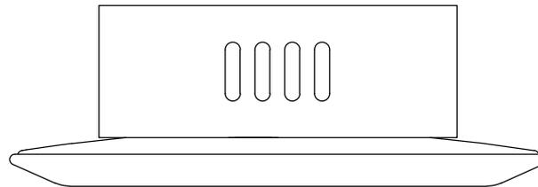
The fixture is designed to dim with a standard Triac forward phase dimmer. Dimming levels will vary by dimmer.
