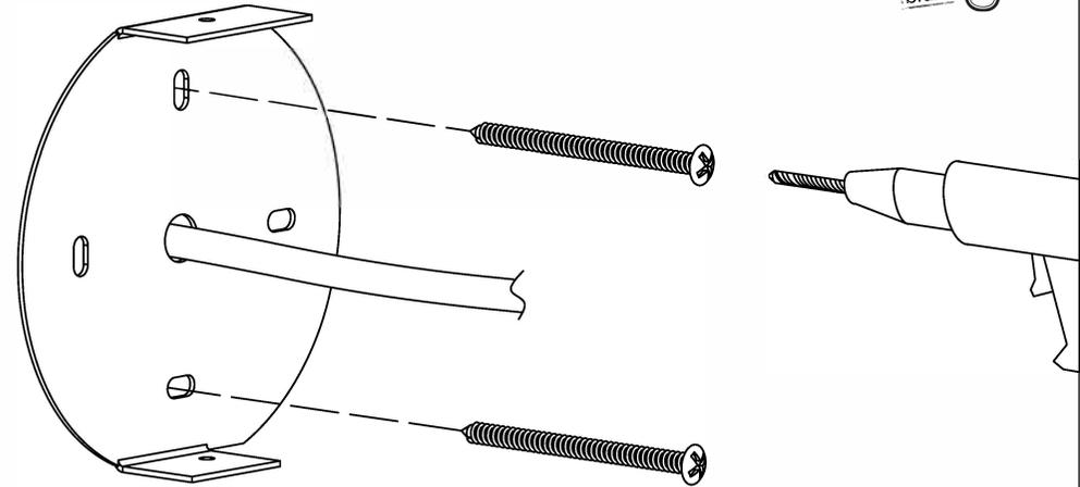
Fix the connector with the cable wired.
