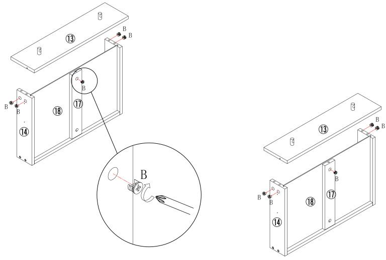
Make sure the arrow on the screw align to the hole on the side.
