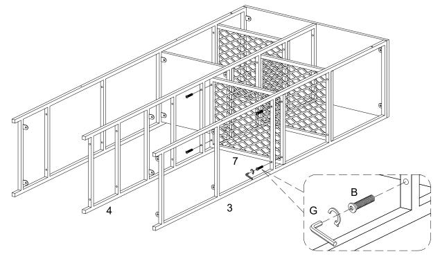
Attach part (7) to part (3,4) using bolt (B) with hex key (G).
