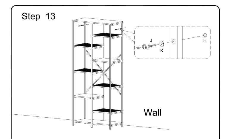
Secure furniture to anchor (H) in wall using washer (K) and screw (J) with a screwdriver.
