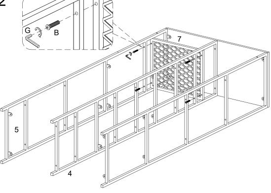
Attach part (7) to part (4,5) using bolt (B) with hex key (G).
