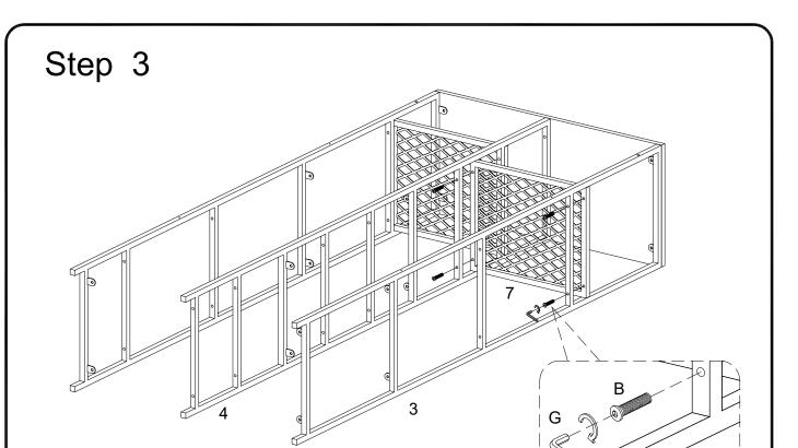
Attach part (7) to part (3,4) using bolt (B) with hex key (G).
