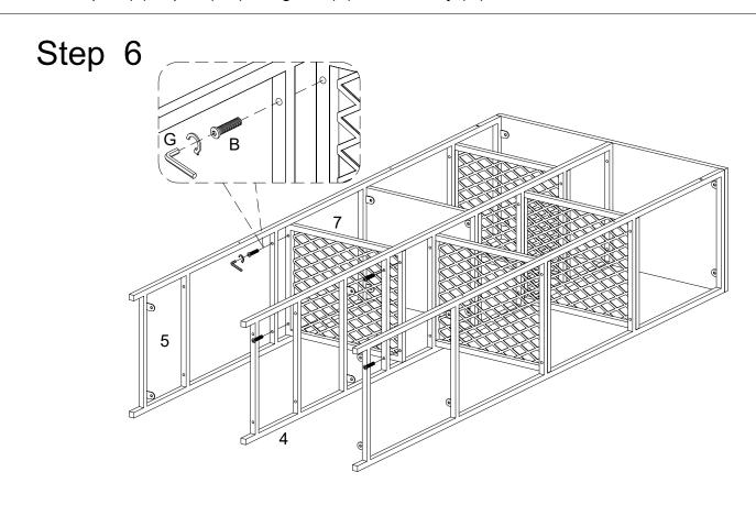
Attach part (7) to part (4,5) using bolt (B) with hex key (G).
