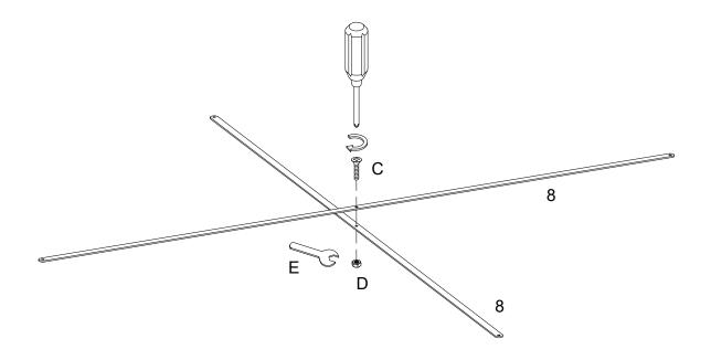
Attach part (8) to part (8) using bolt (C) with a screwdriver and nut (D) with wrench (E).
