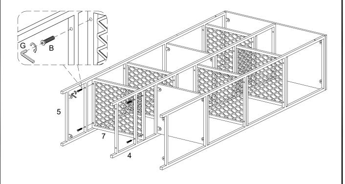
Attach part (7) to part (4,5) using bolt (B) with hex key (G).
