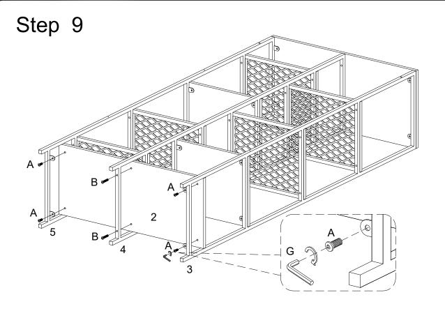
Attach part (2) to part (3,4,5) using bolt (A,B) with hex key (G).
