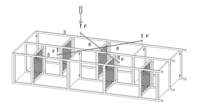
Attach part (8) to part (3,5) using screw (F) with screwdriver.
