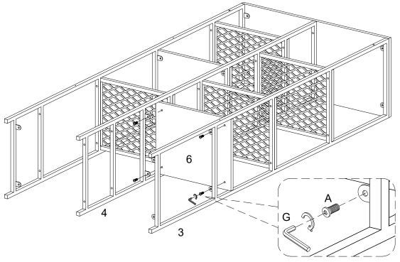
Attach part (6) to part (3,4) using bolt (A) with hex key (G).
