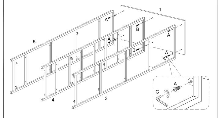
Attach part (3,4,5) to part (1) using bolt (A,B) with hex key (G).
