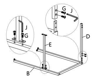
2 Insert Right Frame (C) to Rail (D) and Support Leg (E) using Bolt (G) with Allen Key (J). Note: At this stage, do not fully tighten the Bolts.
