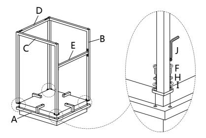
4 With assistance from an adult partner, stand the Stool up. Adjust the Pre-installed Levelers at the bottom of the Left Frame (B) and Right Frame (C) until the Stool levels with the ground.
