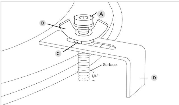
**STEP 5 - ATTACH UNDERMOUNT CLIPS**
