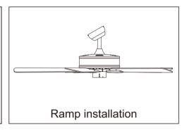
Standard drop ball installation is suitable for general building installation, ramp drop ball installation is suitable for installation on the inclined plane (inverted as inclined roof). The ceiling type installation is suitable for the lower floor space.
