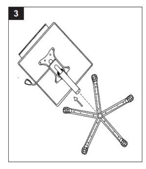
Step 3 Attach leg (B) to seat (A).
