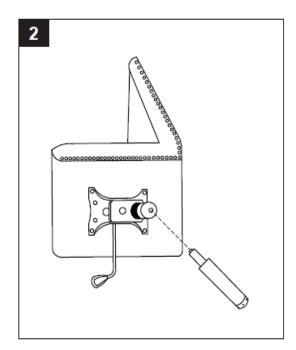
Step 2 Attach Gas Bar (D) to seat (A).
