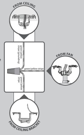
Turn the splices upward and push them carefully back through the hanger bracket into the outlet box. Spread the wires apart, with the grounded wires on one side of the outlet box and the ungrounded wires on the other side of the outlet box.
