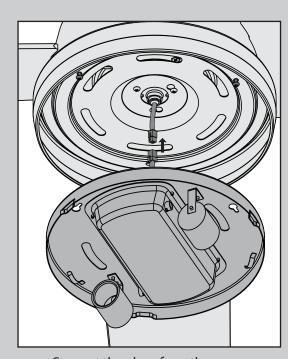
Connect the plugs from the upper and lower switch housings. Make sure to line up the colored markings on the connectors. Wrap light kit keyhole slots around the screws and twist counterclockwise.
