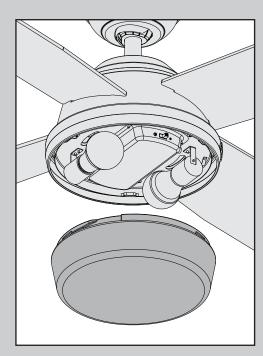
Changing the bulbs - carefully remove the globe. Unscrew bulbs and replace with bulbs of the same wattage. Reinstall the globe.
