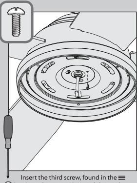
hardware bag, into place and then tighten all three screws.
