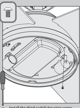
Install the third switch housing screw.
