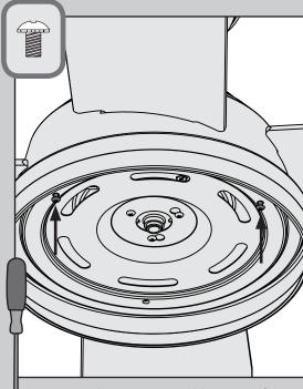
Screw two housing assembly screws from the ≡ hardware bag halfway into the upper switch housing. It does not matter which two screw holes you choose.
