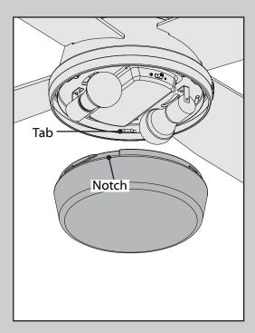
Lift the globe and align the notches in the globe with the tabs in the light kit. Attach the glass bowl to the light kit by twisting it clockwise until it snaps into place.
