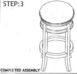
NOTICE:Before assembly screws,have to make sure that legs were keep in a stable position, and then tightening screws,if not, the chairs will be wobble. Even though the stability test passed, but that need to adjust screws, and hold on legs are stable
