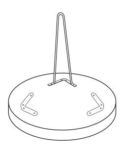
Line up one leg at a time to the holes or marked lines.
