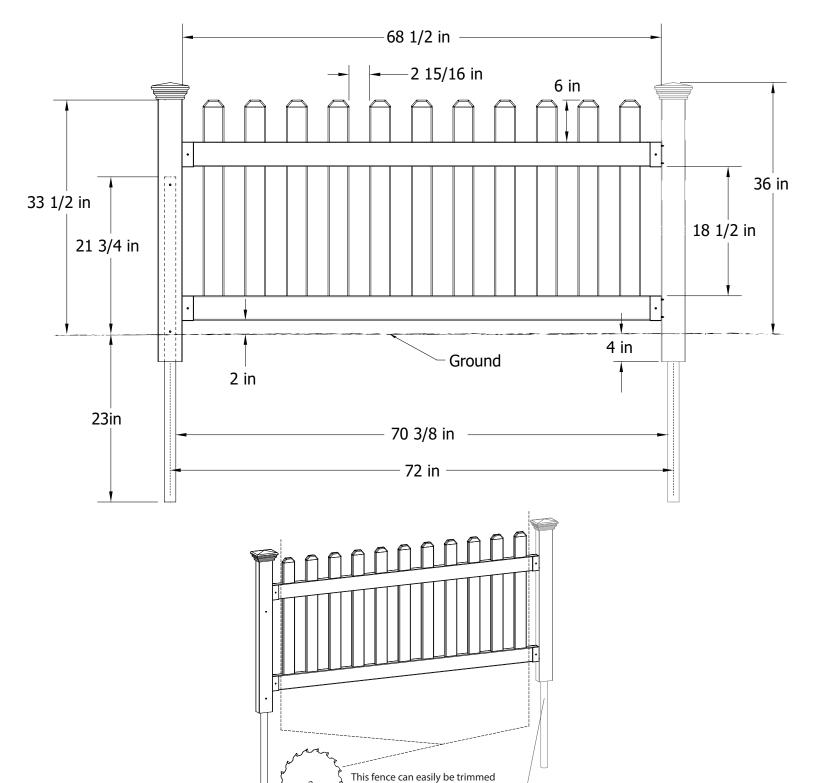
2"x3½" Fence Run Finishing Post with Cap and No-Dig Steel Pipe Anchor Kit Sold Separately
