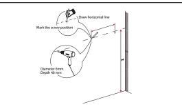
② Install the mirror: use a pencil to mark the placement of the screw holes on the wall, drill the holes and insert the plastic wall anchors.
