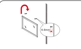
③ Install the screws into the wall anchors, leaving enough of the screw exposed to hang the mirror - approx 1/4" -1/2".
