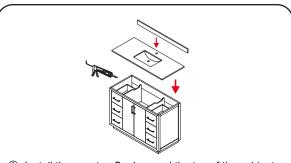
① Install the counter. Seal around the top of the cabinet with clear silicone sealant. Do not over apply. Allow to dry 24 hours for proper curing.
