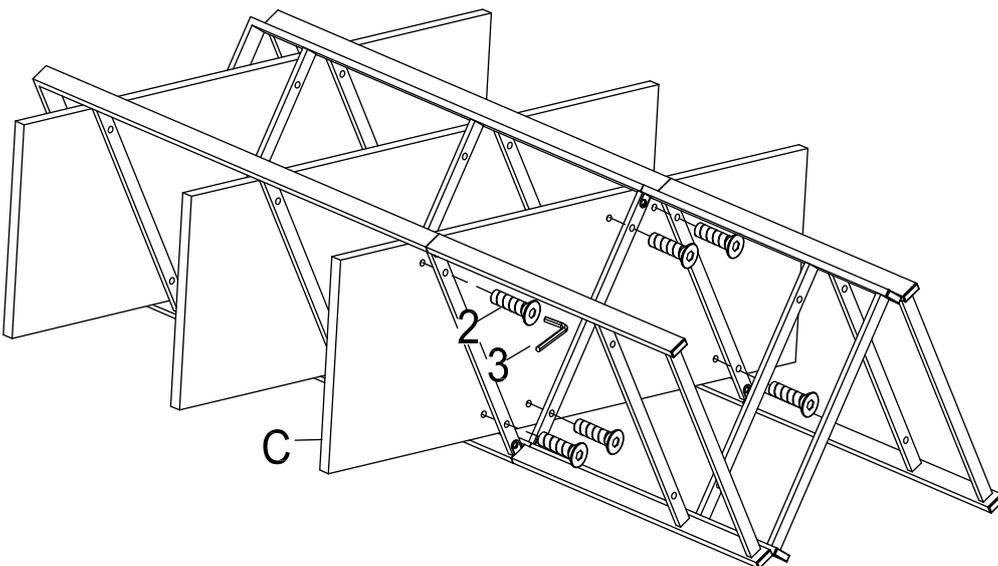
Attach the wood shelf (C) to the assembled unit using bolts (2) as shown.
