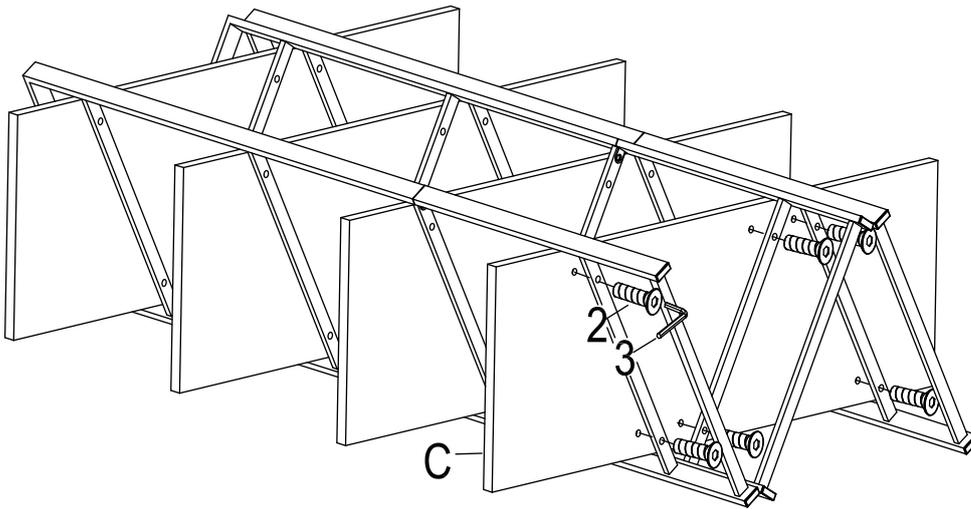
Attach the wood shelf (C) to the assembled unit using bolts (2) as shown.
