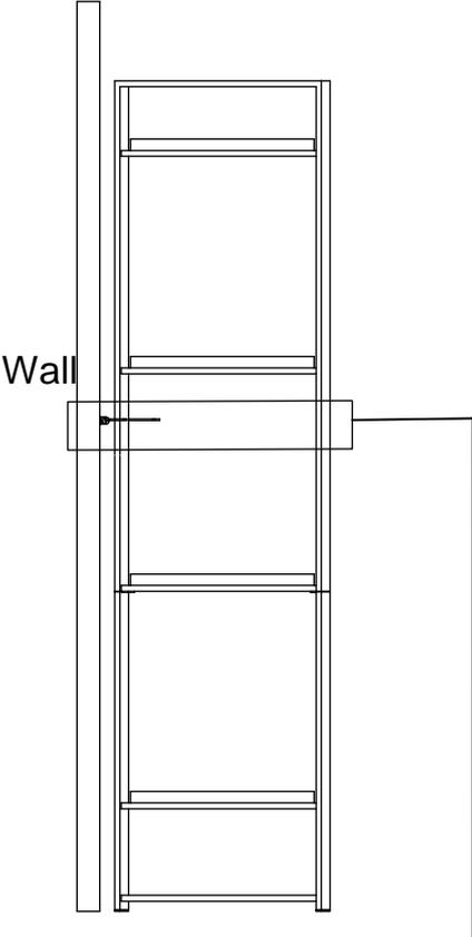
Insert each end of the plastic strap (7) into L brackets (5), then secure and tighten.
