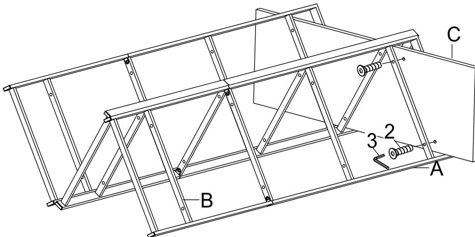
Attach the large side panel (A) to wood shelf (C) using bolts (2).
