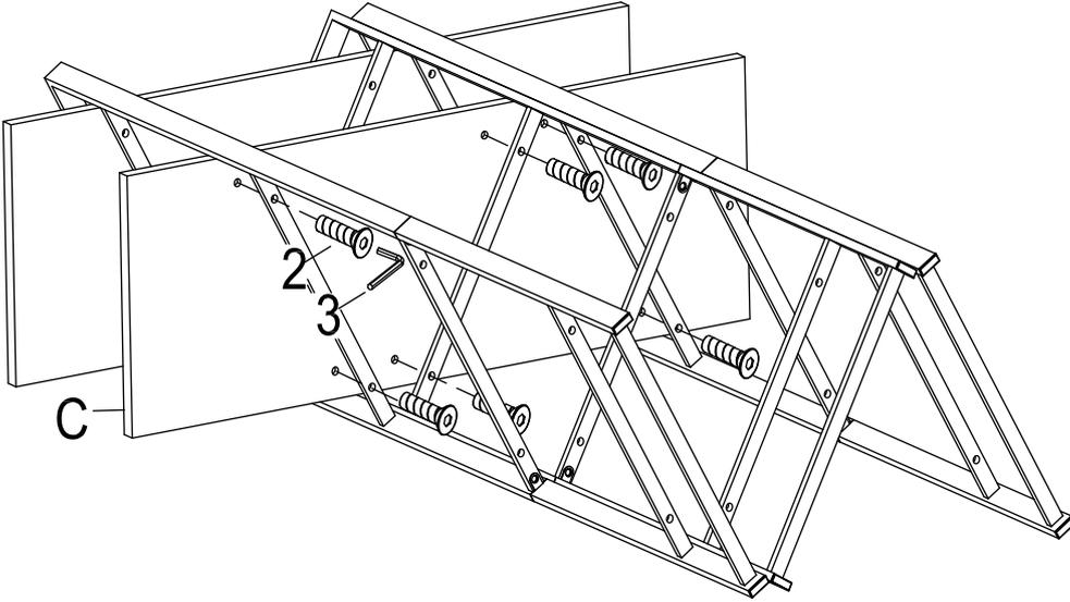
Attach the wood shelf (C) to the assembled unit using bolts (2) as shown.
