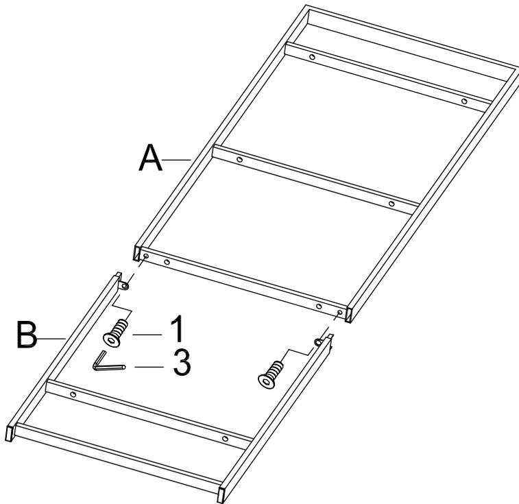
Attach large side panel (A) to small side panel (B) using bolts (1) as shown.
