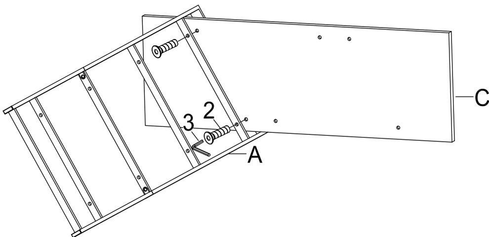
Attach wood shelf (C) to one large side panel (A) using bolts (2) as shown.
