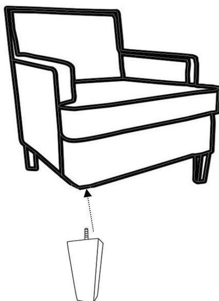
Step 1: Take out two front feet and two back feet from the carton and put into the screw holes underneath the base and screw tight to the right angle.
