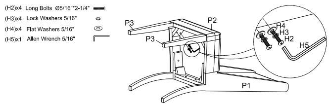
Step 4. Securely tighten all bolts with Allen wrench (H5), but do not over tighten the bolts. Turn the assembled chair to upright position. Make sure the chair is level. Assembly is complete. **Failure to follow these unstructions may cause the bolts to misalign during assembly.**
