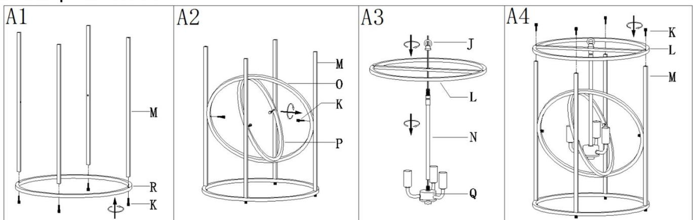
**Step A1:** Fix the tubes (M) to the lower iron ring (R) with screws (K).
