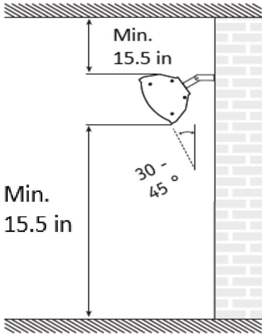
The heater must be installed at least 6 feet above the floor
