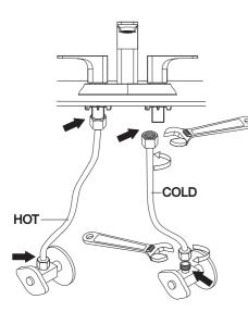
3. Connect the water supply lines to the tail pipes of the faucet and to the hot and cold water supply valves. Secure and tighten with an adjustable wrench. Caution: Be careful not to mix up the hot and cold supply lines.
