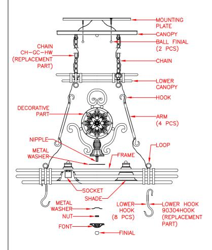
AVAILABLE PARTS ARE: CH-GC-HW (CHAIN) 90304HOOK (LOWER HOOK)
