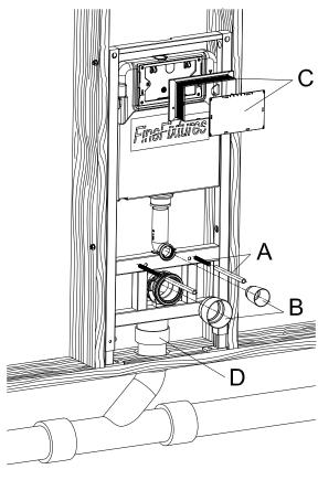
A Install M12 rods with plastic sleeves, B pipe plugs and C mud guard during the rough-in installation
