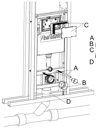
A Install M12 rods with plastic sleeves, B pipe plugs and C mud guard during the rough-in installation
