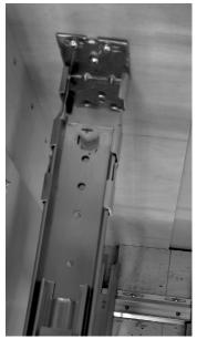
Remove the unit from the base again and then slide the rear mounting bracket off the slide. Align the rear bracket prongs with the indentation marks on the rear of the cabinet and secure with three (3)  $\#8 \times 5/8$ " Pan Head Wood Screws in the slots as shown. Re-install the unit onto the slides, making sure as you push it in the cabinet, that the top slide is properly seated into the rear mounting bracket. Operate the unit to make sure the undermount slides are working properly.
