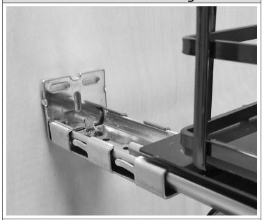
If the countertop is installed, pull the organizer partially open to gain access to the upper slide. Firmly grasping the upper slide, tap it against the back of the cabinet. The rear bracket should make small indentations in the back of the cabinet. Proceed to step 4. If countertop is not installed, pull the organizer partially out to gain access to the rear bracket and install three (3) #8 x 5/8" Pan Head Wood Screws provided in the slots. Proceed to step 5.
