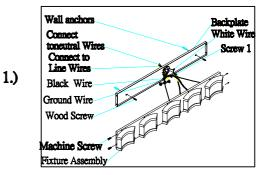
Step.1: remove mounting bracket (A) from fixture (C) and install it to electrical box.
