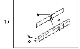
Step.2: Install fixture to back-plate and tighten screws (B) so that fixture meets the wall.
