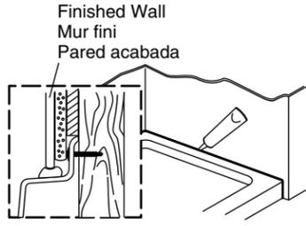
**17** Install the finished floor. Apply 100% silicone sealant along the floor seam.
