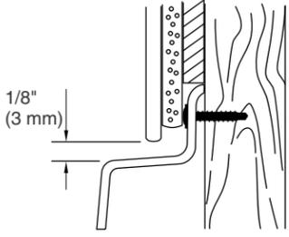
**16** Apply 100% silicone sealant around the shower base where it contacts the finished walls.
