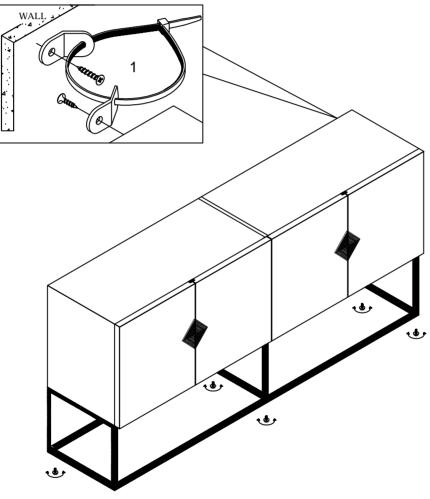
Adjust levelers if needed to level case on uneven floor.
