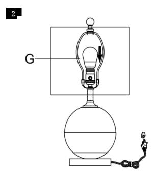
Step2 Insert the bulb( G) into the socket(C).
