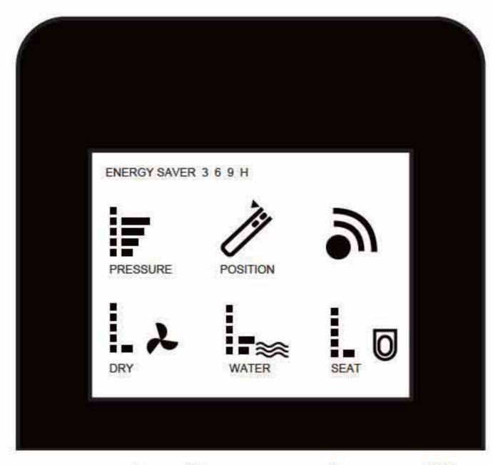
For example, the nozzle position is on level 2, and massage function is open; the water pressure is on level 4; water temperature is on level 2, while dry temperature and seat temperature are on level 1.
