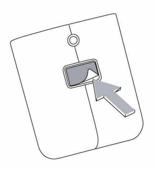
(3)Insert expansion tube into the hole on the wall, install the hanger to the wall with a screw, and paste the double faced adhesive tape on hanger to the wall, tighten the screw.
