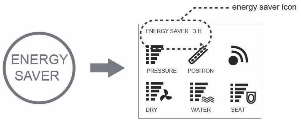
(2)Press"ENERGY SAVER"button again, LCD screen shows figure "6", and the "ENERGY SAVER"icon disappear after 3 seconds, the setting succeeds. The toilet enters the energy saver mode from 9:00 to 15:00 every day. During this period, power light is off, and the energy saver light is on. It goes back to normal operation mode after energy saver time.
