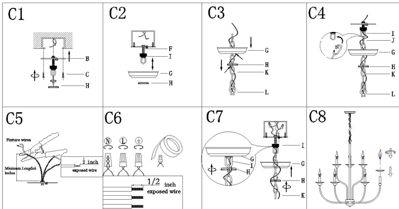
Step C1: .Attach single bar (B) to outlet box with mounting screw (C). The side of single bar marked "GND" must face out.
