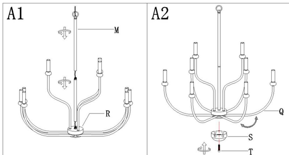
Step A1: Carefully thread stem (M) onto the top of wire house (R) until snug .
