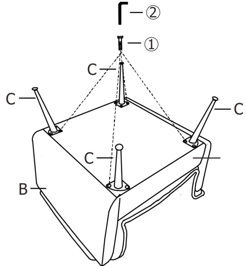
STEP 1 : Use bolt ①, allen key ② to attach legs B
