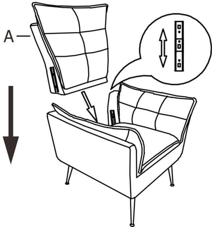
STEP 2: Carefully align male and female metal bracket then push all the way down to secure.
