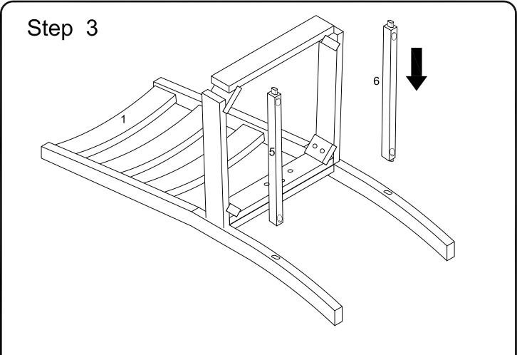
Insert support bar (5,6) into back frame (1).
