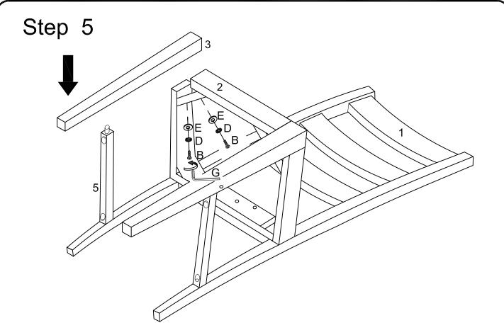
Insert leg (3) into support bar (5), use wrench (G) to secure seat frame (2) to leg (3) with bolt (B), spring washer (D) and washer (E).
