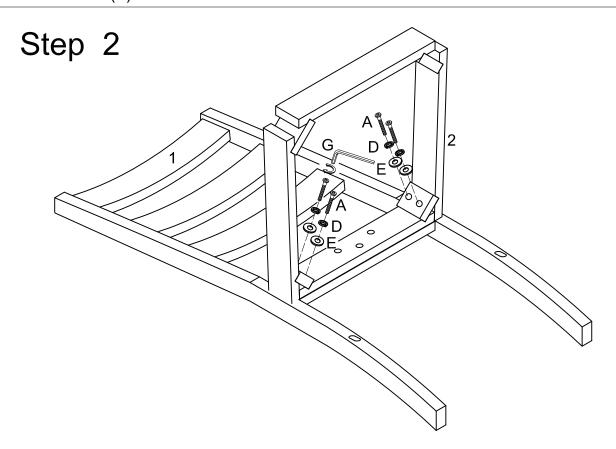
Use wrench (G) to secure seat frame (2) to back frame (1) with bolt (A), spring washer (D) and washer (E).
