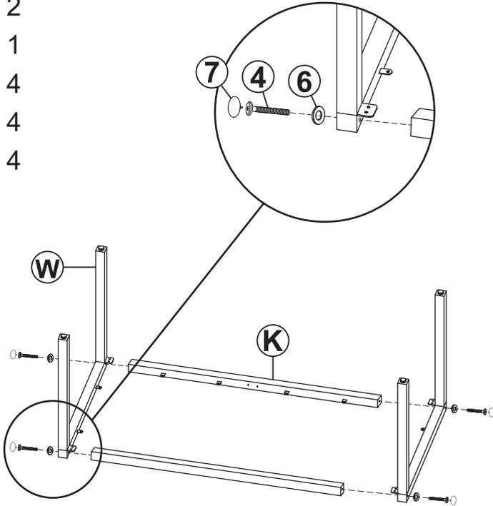
Do not fully tighten hardware until after Step 8 is complete.
