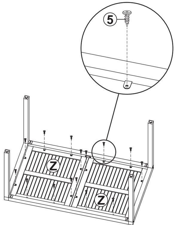
Fully tighten all table hardware after this step is complete.
