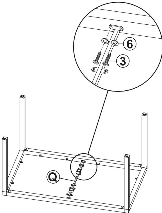
Do not fully tighten hardware until after Step 8 is complete.
