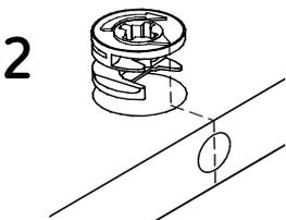
You should insert these cams with the little arrow pointing towards the drilling on the panel's edge (shown on the left).
