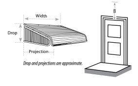
Standard sidewings require 13" of mounting space over door (B). Low-mount sidewings require 6" of mounting space over door.
