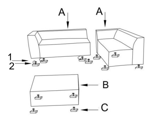
Attach the Feet (C) using Washers (1) and Screws (2) to each corner of the Loveseat (A) and Ottoman (B).
