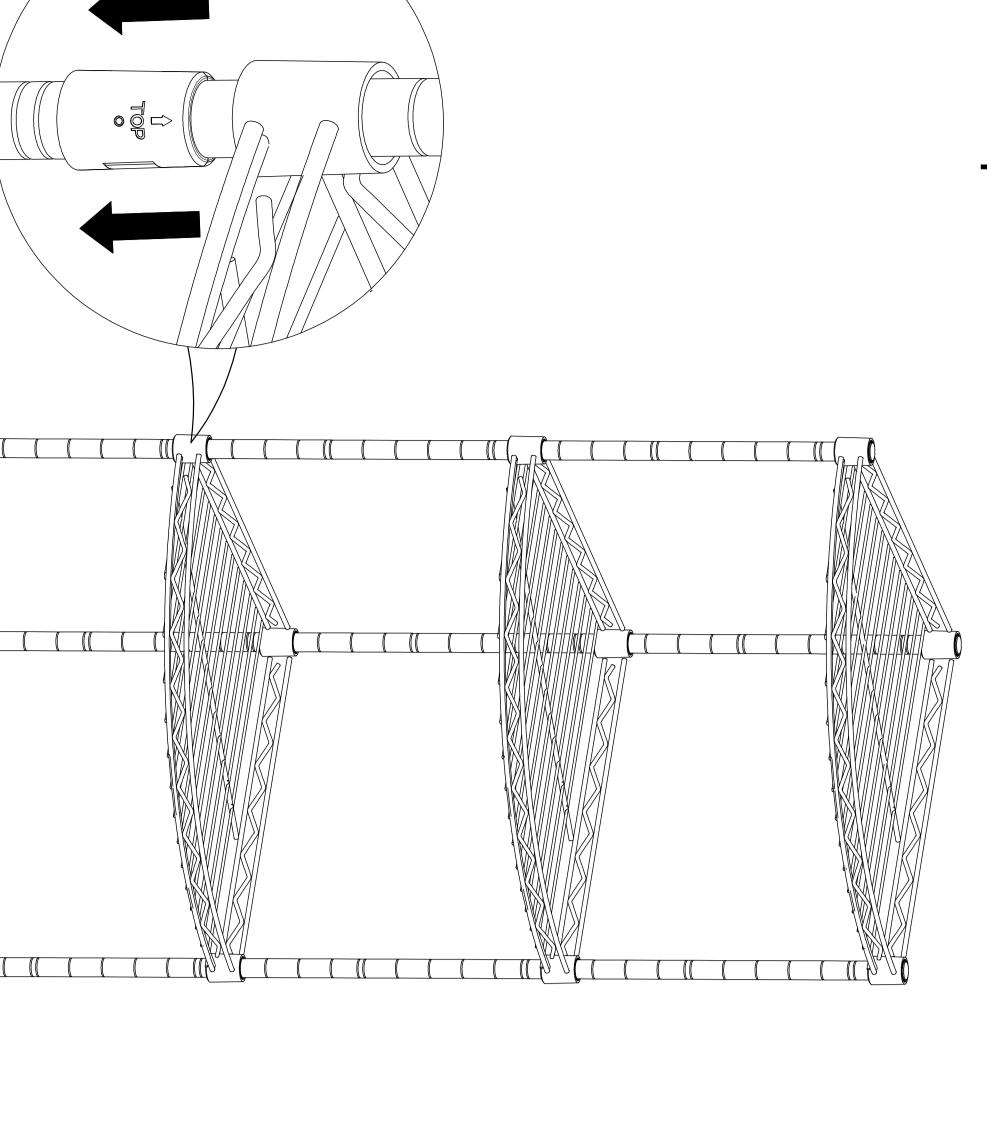
Assemble the short leg(D) by screw bracket(E) onto the bottom fan-shaped shelf at the middle of curved snake area as the photo.
