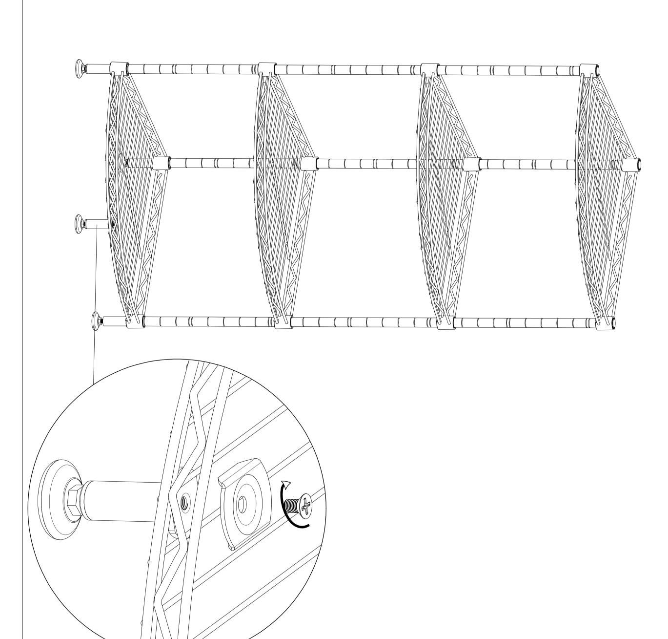
Pushing firmly down on every fan-shaped shelf at corners by rubber mallet to ensure all the fan-shaped shelves in a place over the plastic clips. And screw leveling feet in or out to attain proper leveling.
