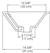
By IAPMO, ceramic lavatory warpage is defective only if warpage of flat slab out of horizontal plane exceeds 6.3 mm/m (0.25 in/ft) on all sizes OR warpage on back of lavatories that are attached to the wall exceeds 3 mm (0.13 in).
