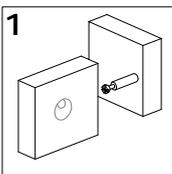
1: Insert Cam Bolt into bolt holes on the flat side. Don't over tighten!
