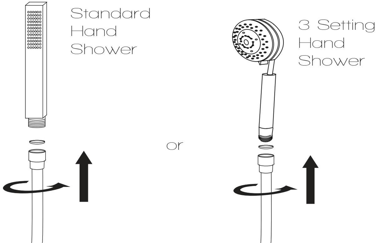
**Step 2A** Finally, install the hand shower to the hose, as shown.
