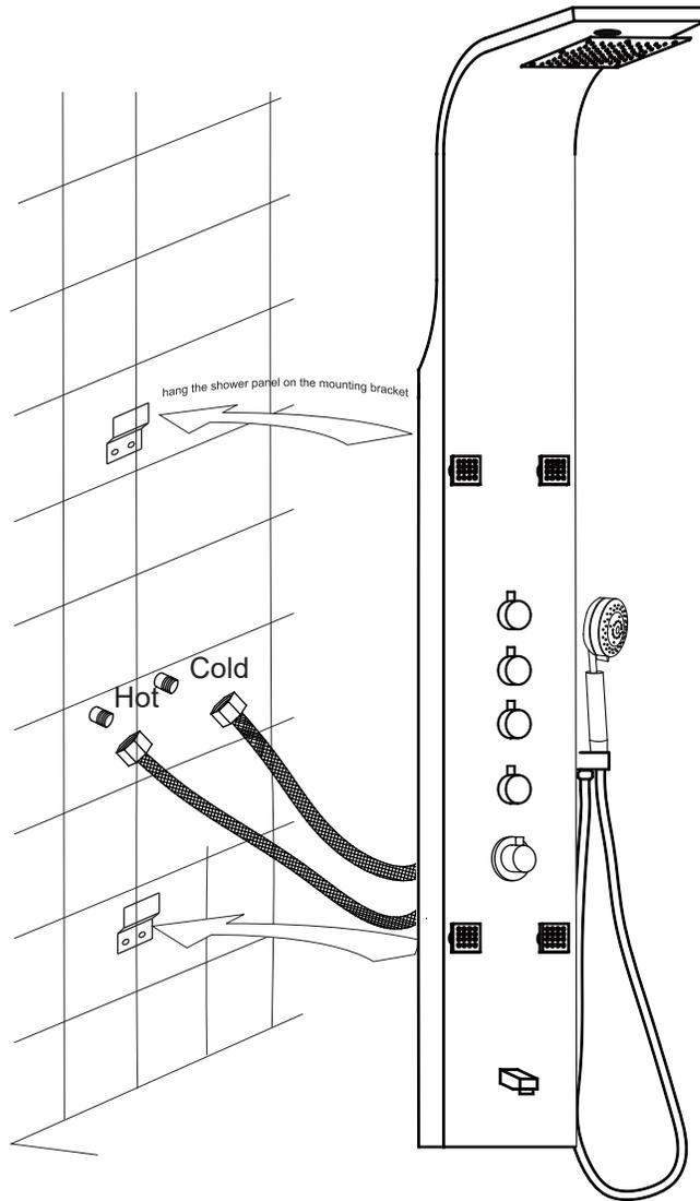
**Step 4A** Screw the cold and hot water hose from the shower panel to the supply lines in the wall.
