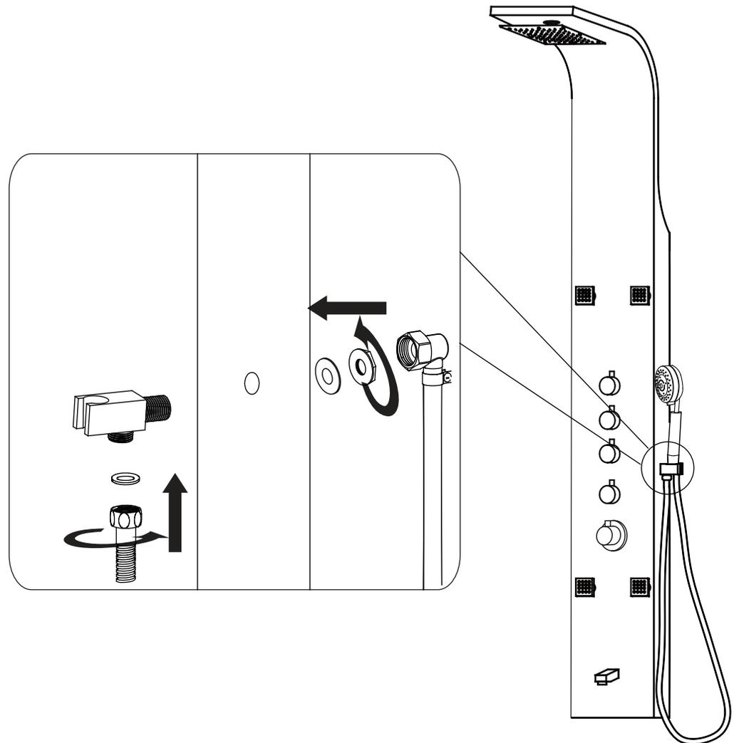
**Step 1A** Insert the hand shower holder through the pre-drilled hole on the shower panel.
