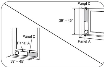
For window openings from 39" to 45", use the window vent panel (Panel A) and an extension panel (Panel C).
