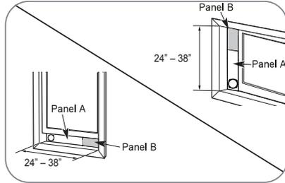
For window openings from 24" to 38", use the window vent panel (Panel A) and an extension panel (Panel B).
