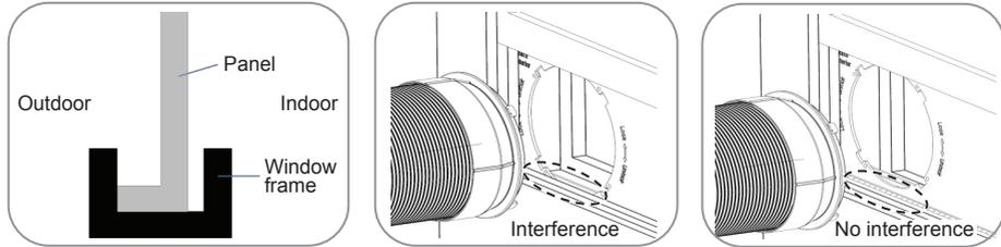
**To install hard foam shims:** If any extension panels are used, attach foam seal(s) H to the bottom side of extension panel B or C to minimize gaps. Then attach the hard-foam shim(s) G along the bottom side of the window panel assembly to allow the vent hose to clear the window frame. (See image in step 3.)
