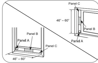
For window openings from 46" to 60", use the window vent panel and two extension panels (Panel B and Panel C)
