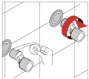
**2.** Connect the installation adapters to the water supplies. Use a small amount of teflon tape to ensure a watertight seal.
