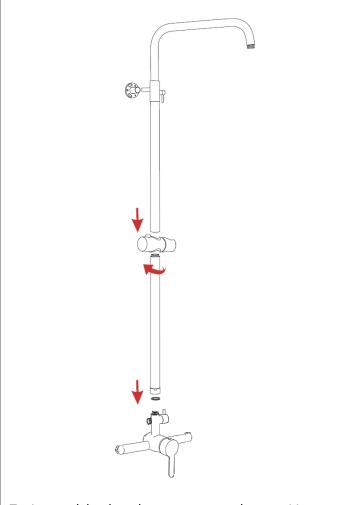
**5.** Assemble the shower set as shown. Use sealing washers where needed.
