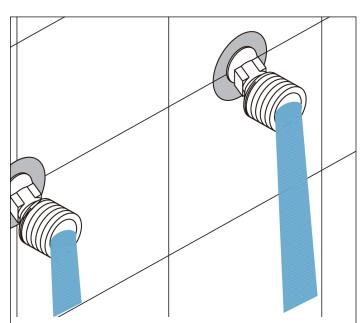
**4.** Turn the water on for several minutes to flush the supply lines. This will prevent dirt and impurities from entering the cartridge and reducing water pressure.
