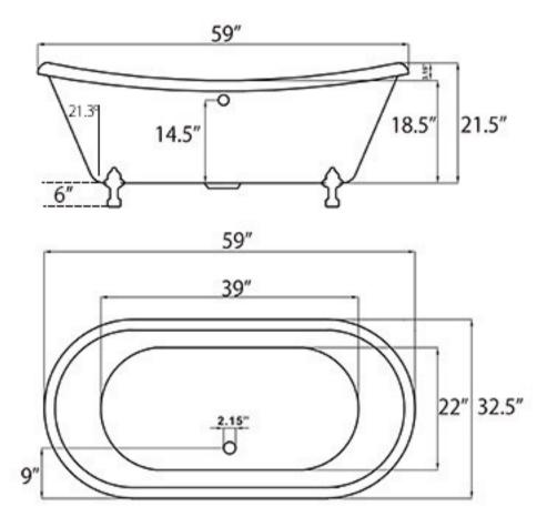
This tub has an integrated drain overflow, drain tail piece to floor will fit directly from under the tub drain position noted on the drawing
